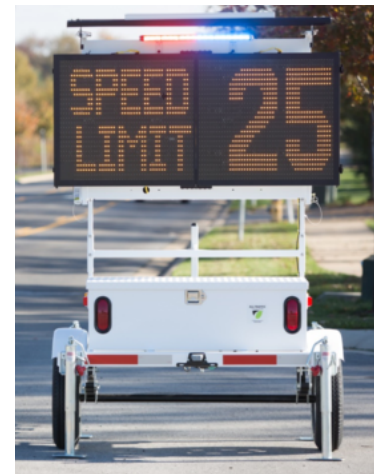
SpeedAlert 24 on an ATS 5 Trailer
