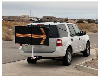
InstAlert 24 on a hitch mount
