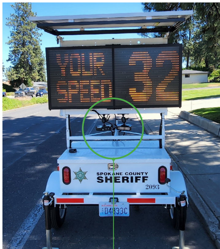
CAMERAS MOUNTED UNDER SIGN
