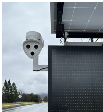
Camera mounted to trailer arm
