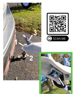
G. Back the vehicle up to the trailer so that the hitch ball (2) is just in front of the coupler (1). If necessary, have a partner guide you or use a backup camera if it provides a clear view. When your vehicle is in position, shift into park, apply the parking brake, and turn off the engine.
