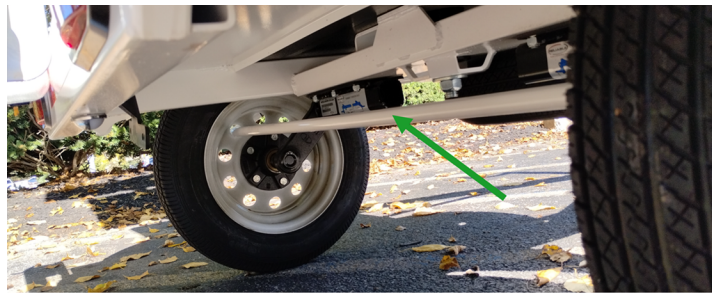
Figure 11, The axle lock bar installed
