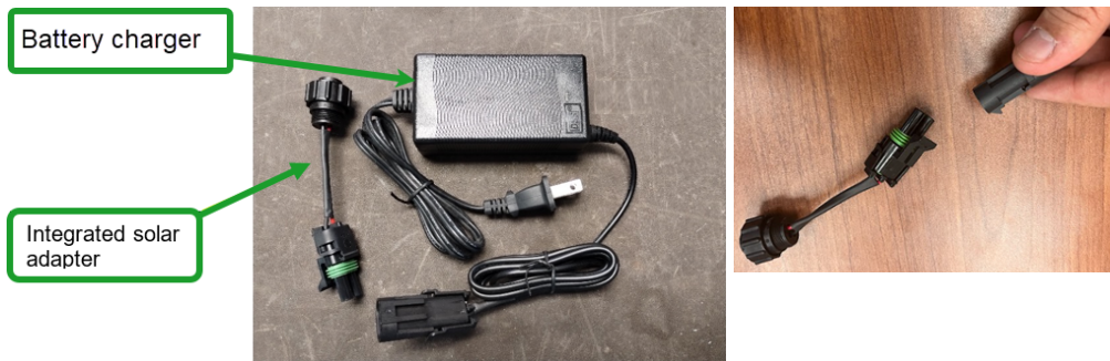
Figure 12, Connecting the charger cable to the solar adapter dongle
