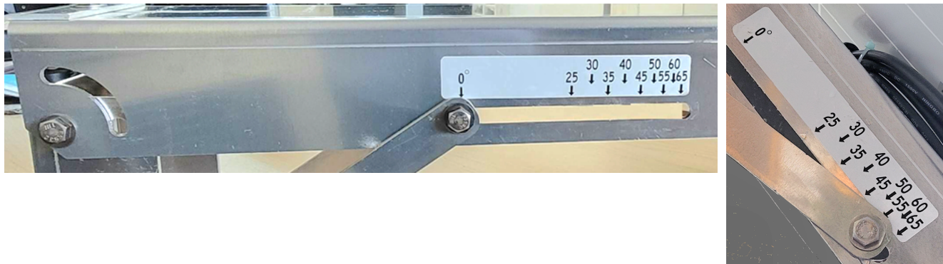
Figure 10, The solar panel angle gauge
